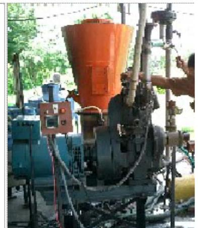
**Figure 9:** Small scale gasifier-engine in India (Source: ANKUR 2003)
